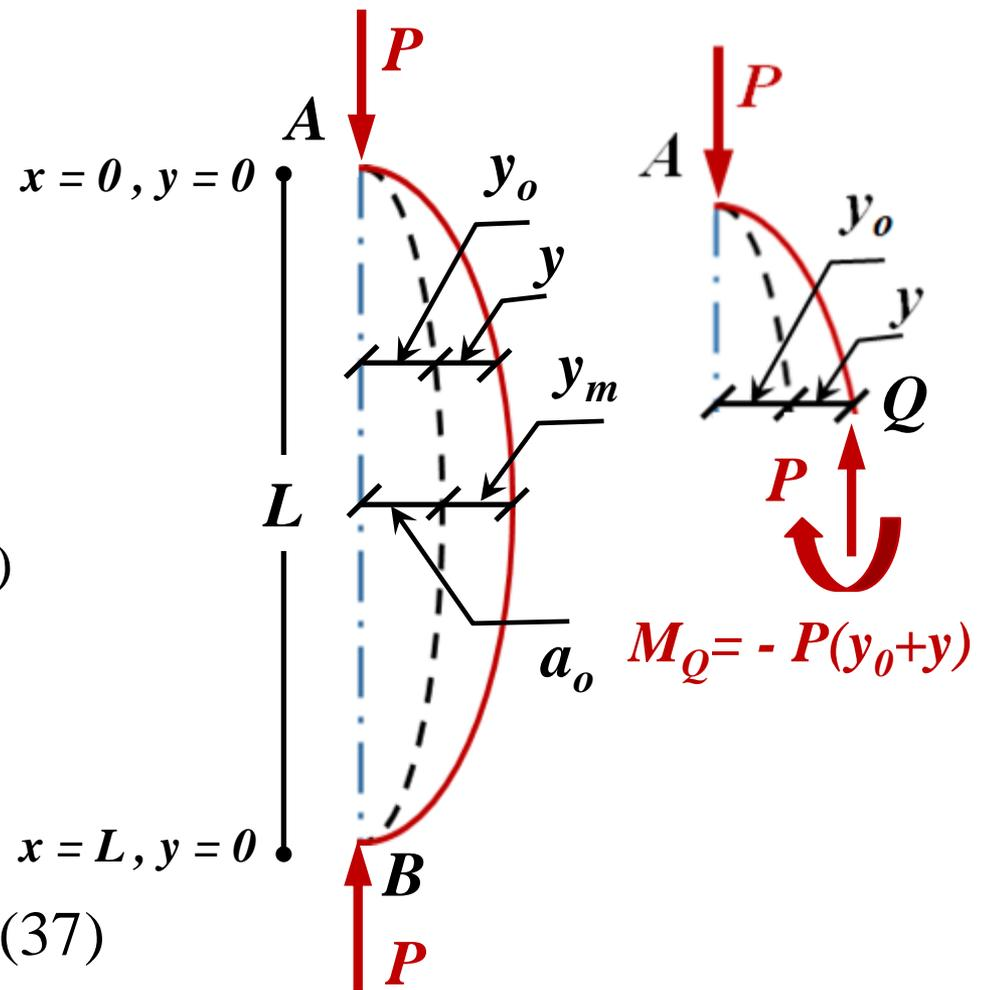
$y_0$  = initial deviation of the column and is represented by the sinusoidal curve
