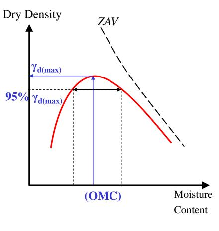
Relative compaction, or percent compaction is defined as the ratio of the  $(\gamma_d)_{\text{field}}$  to  $(\gamma_{d \text{ max}})_{\text{lab}}$ .
