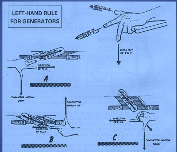
A useful convention also exists that a conductor shown as  $\oplus$  means that the current is flowing *away* from the observer, whereas one shown as  $\odot$  means that the current is flowing *toward* the observer. This convention will be used from now on.
