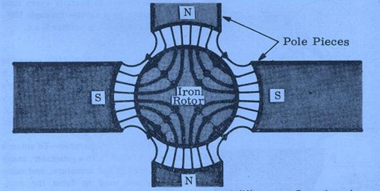
The generator can clearly be arranged in several different configurations, just so long as the principle of *conductors cutting through magnetic fields* is preserved. You will meet some of these different configurations later on in this Part 5 of *Basic Electricity*.
