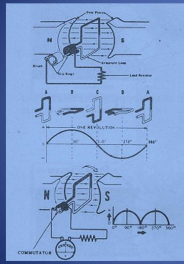
3. The Elementary Generator—A loop of wire rotating through a magnetic field forms an elementary generator when it is connected to an external circuit through slip rings. The induced e.m.f. causes current to flow in the external circuit.
