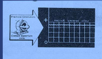
6. Practical D.C. Generator—To smooth out the d.c. taken from a generator, many coils are used in the armature, and more segments are used to form the commutator. A practical d.c. generator produces a voltage output which is near maximum at all times, and which has only light ripple.
