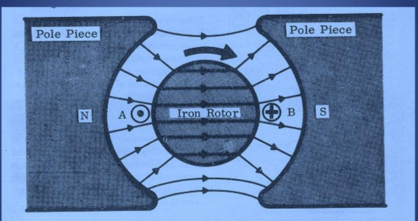
The flux can be made greater and even more uniform by using more than one pair of poles. Two pairs of poles are common, but more may be found in use in large machines.
