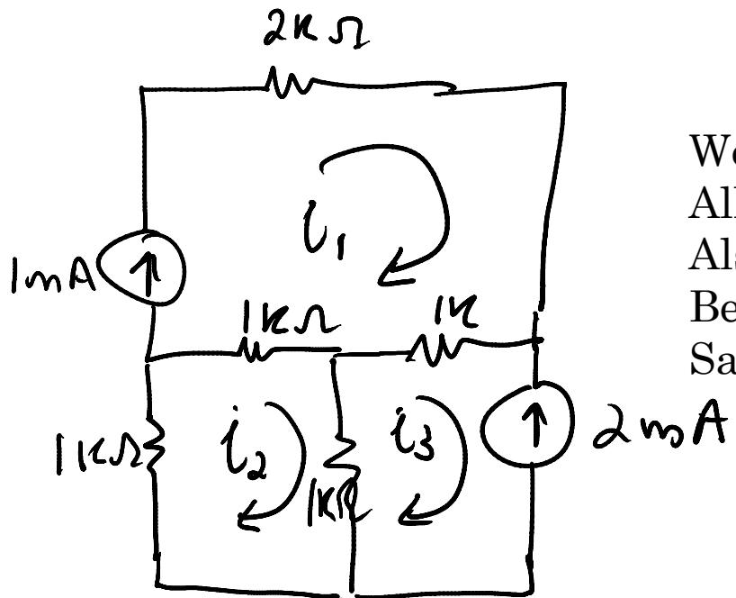
We simply assume clockwise current flow in All the loops and find them to analyze the circuit. Also any independent current source in a loop Becomes the loop current as current in series is Same.
