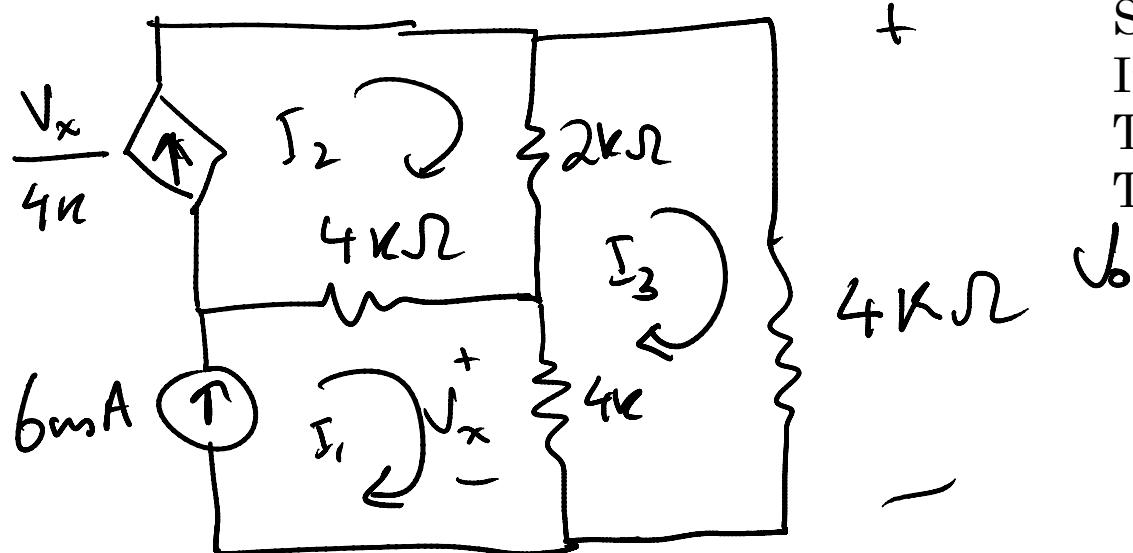
Simplify the circuit using the Independent sources by assigning Them to the mesh currents for The specific loop.
