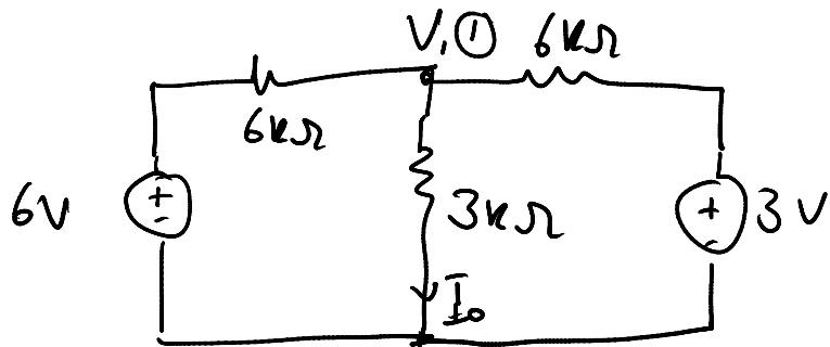
$$\frac{V_1 - 6}{6\text{k}} + \frac{V_1}{3\text{k}} + \frac{V_1 - 3}{6\text{k}} = 0$$
