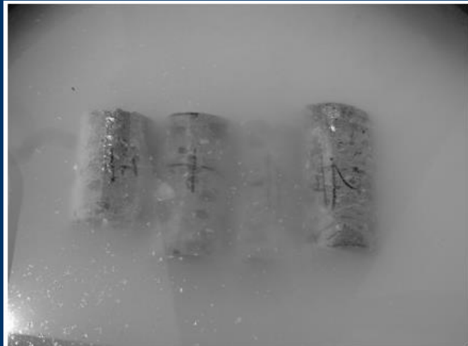
Fig. Core Samples Dipped in Lime Water
