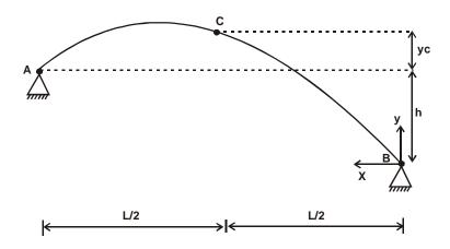
11.5. Derivation for center-line of a parabolic arch with supports at different levels.
