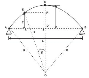
As span and central rise are usually known, Radius of arch R can be calculated from (9)
