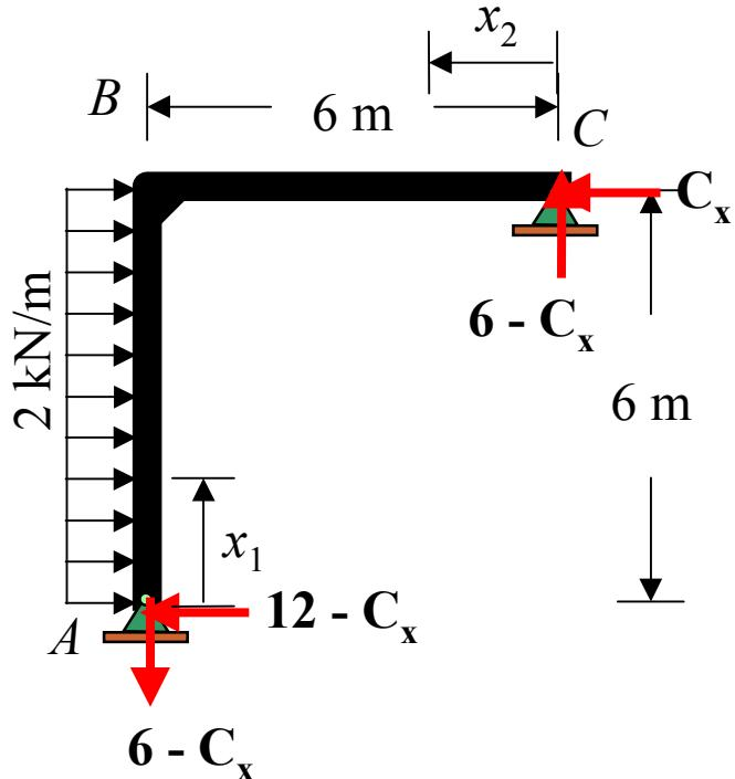
$$\frac{\partial U_i}{\partial C_x} = \int_0^L \left( \frac{\partial M_i}{\partial C_x} \right) \frac{M_i}{EI} dx = \Delta_{CH} = 0$$
