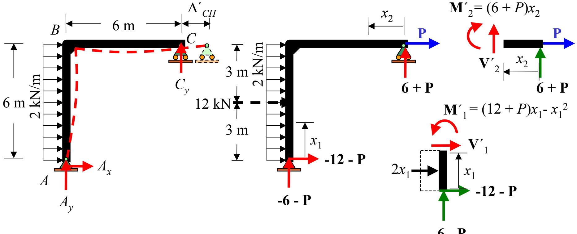
$$\begin{aligned}\Delta'_{CH} &= \int_0^L \left( \frac{\partial M'_i}{\partial P} \right) \frac{M'_i}{EI} dx = \frac{1}{EI} \int_0^6 (x_1)(12x_1 + x_1^2 - x_1^0) dx_1 + \frac{1}{EI} \int_0^6 (x_2)(6x_2 + x_2^2 - x_2^0) dx_2 \\ &= \frac{1}{EI} \int_0^6 (12x_1^2 - x_1^3) dx_1 + \frac{1}{EI} \int_0^6 (6x_2^2) dx_2 \\ &= \frac{1}{EI} \left( \frac{12x_1^3}{3} - \frac{x_1^4}{4} \right) \Big|_0^6 + \frac{1}{EI} \left( \frac{6x_2^3}{3} \right) \Big|_0^6 = \frac{972}{EI}, \rightarrow\end{aligned}$$
