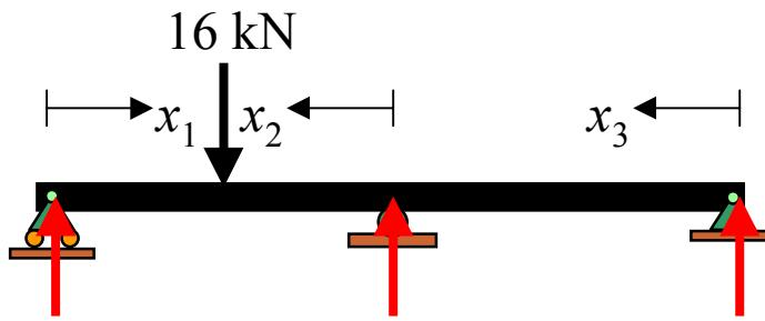
$$R_A = 12 - 0.5R_B \quad R_B \quad R_C = 4 - 0.5R_B$$
