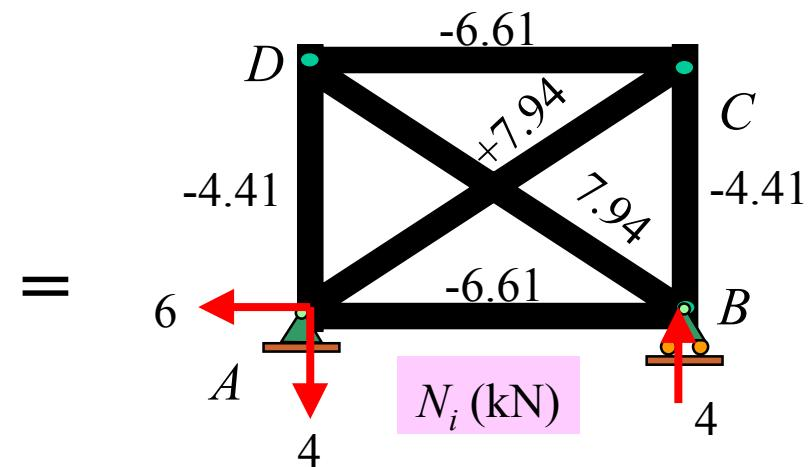
**Part (c) :** If the horizontal force  $P = 6 \text{ kN}$  is applied at joint C and the turnbuckle on member AC is used to shorten the member by 1 mm are both accounted.
