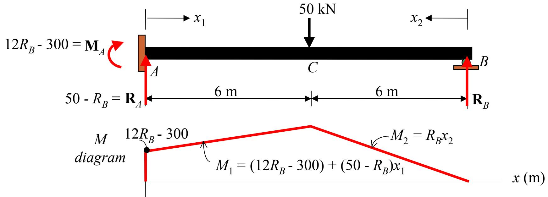
$$\Delta_B = 0 = \int_0^L \left( \frac{\partial M}{\partial R_B} \right) \frac{M}{EI} dx$$
