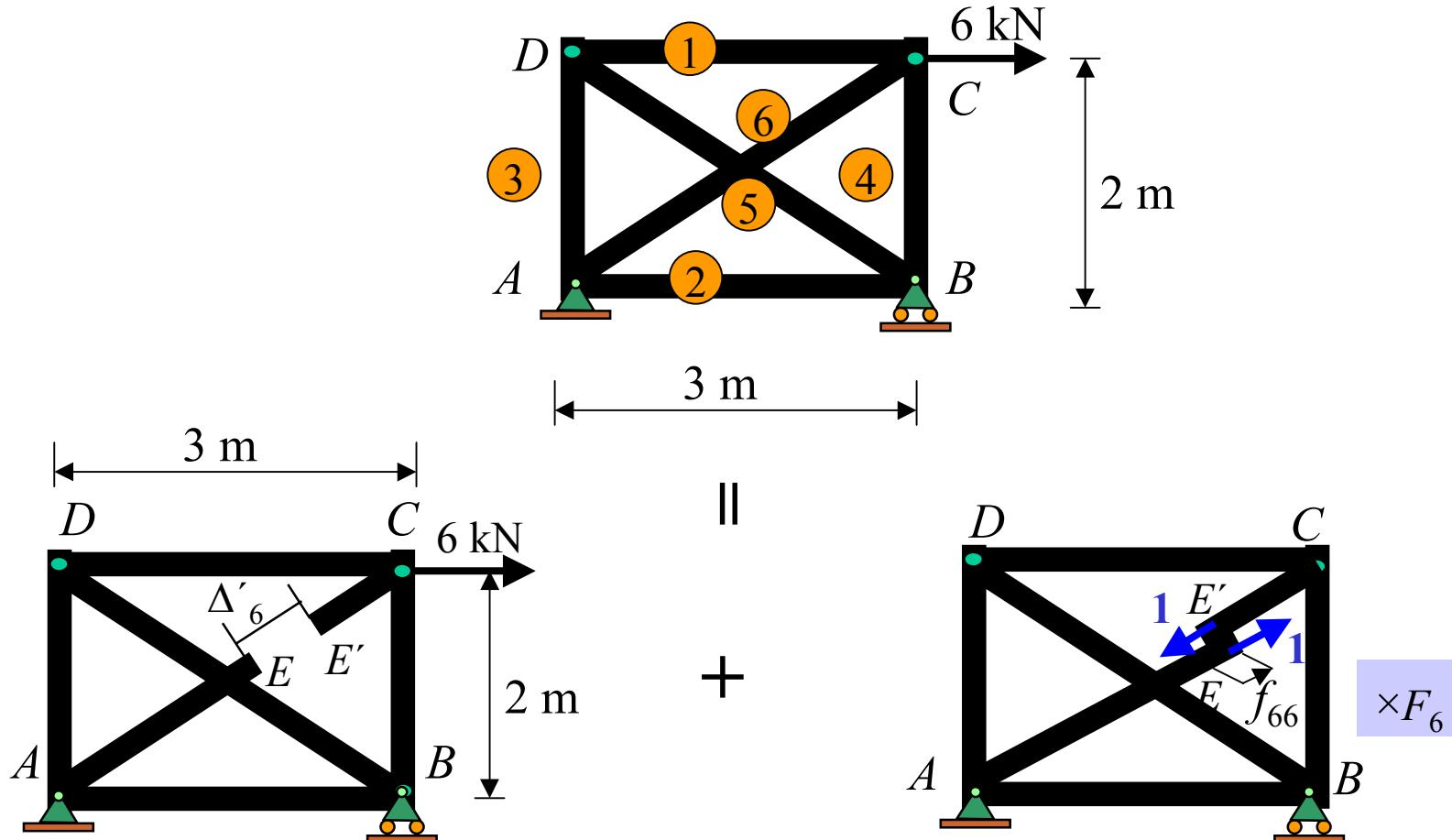
$$\text{Compatibility equation : } \Delta'_6 + f_{66} F_6 = 0 \quad \text{-----(1)}$$
