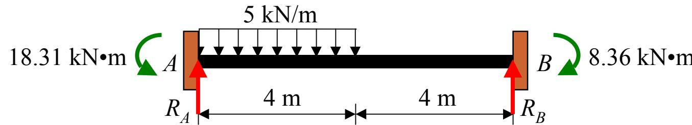
$$+\curvearrowright \Sigma M_A = 0: \quad 18.31 - 20(2) + R_B(8) - 8.36 = 0, \quad R_B = 3.76 \text{ kN}, \quad \uparrow$$
