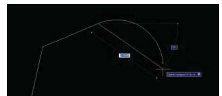
If you type “s” while drawing an arc segment, you can define an arc angle by specifying three points that the arc goes through.
